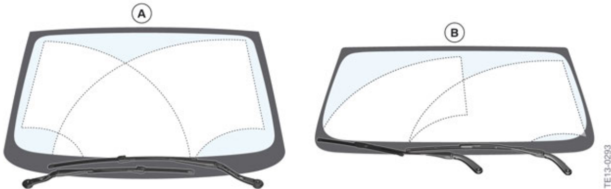
Comparison of wiping pattern of I01 and F30
